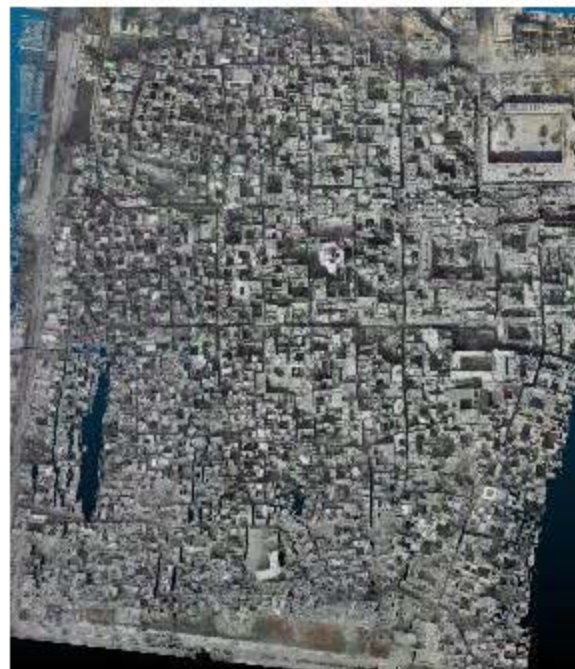
Fig. 67 The Drone-Point-Cloud data before adding any supplementary data set, rendered in Cloud Compare, by Orabi, 2023.
