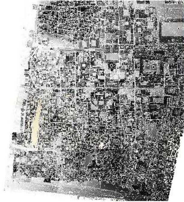
Fig. 105 Mass and void interpreted according to heights, from the point cloud, generated in Cloud Compare, by Orabi, 2023.
