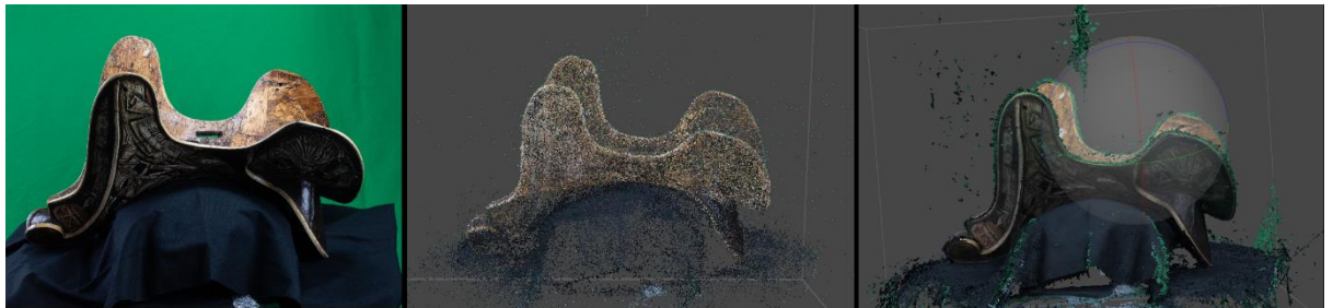
Figure A. 3: Phase photos of the photogrammetry of the London-2: a) single photo example, b) point cloud representation c) 3D mesh. Photo by author.
