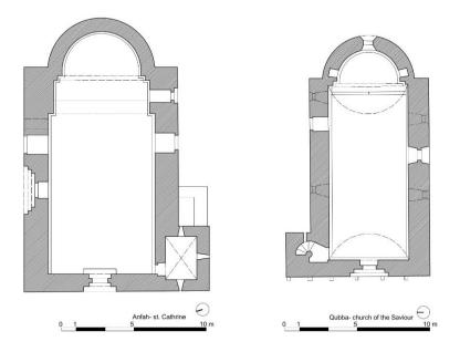
Fig. 74- Floor plan of St Catherin church 'Anfah and the floor plan of St. Saviour church Qubba drawn by the author.
