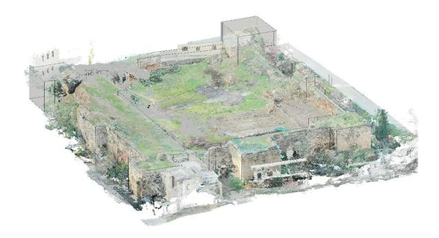
Fig. 87-Reconstruction of the Qulay at castle done on Revit based on the generated point cloud.
