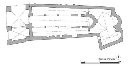
Fig. 77- Floor plan of Mār Jirjis church, Rāshkīdā, drawn by the author based on the drawings published by  $\rm NL$
