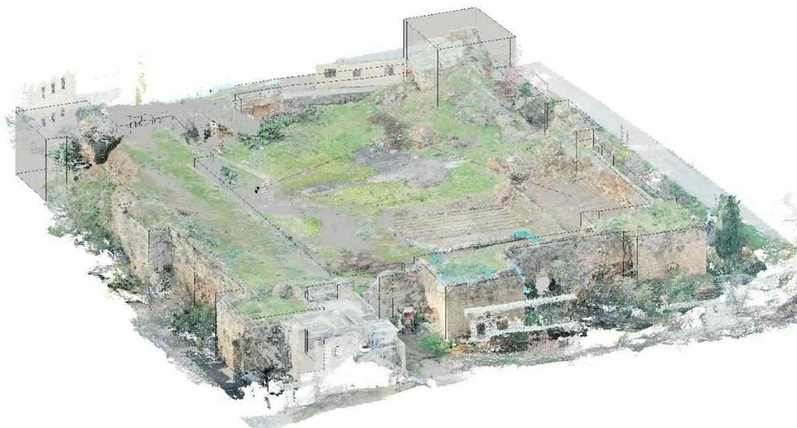
Fig. 87-Reconstruction of the Qulay'āt castle done on Revit based on the generated point cloud.
