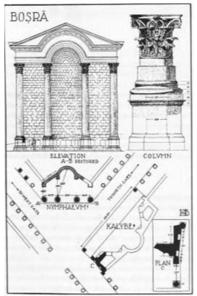
Plate 7: Bosra, the *nymphaeum*, plan and elevation suggested reconstruction. Extracted from: Segal 1997.
