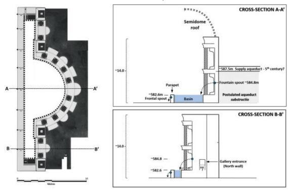
Plate 34: Cross-sections showing water flow through the *Nymphaeum in Gerasa* (Jerash Water Project). Retrieved from Boyer 2022.
