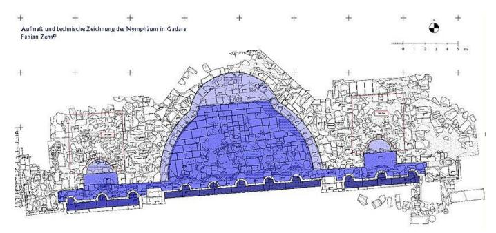
Plate 37: measurment and technique of water distribution within the *nymphaeum* of Gadara source, wetted areas of the *nymphaeum* dark blue lowest heigh of street level, light blow highest of street level. Source (<u>http://www.qanat-firaun.de</u> entered August 2023)
