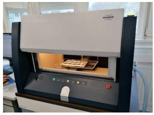
Fig 9: The Micro-XRF Spectrometers M4 Tornado (Photo: Al Halabi Suleman 2021)
