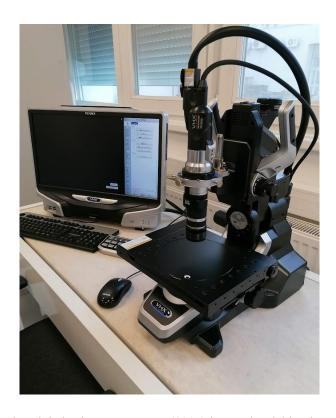
Fig 11: The Digital Microscope VHX-6000 (Photo: Al Halabi Suleman 2021)
