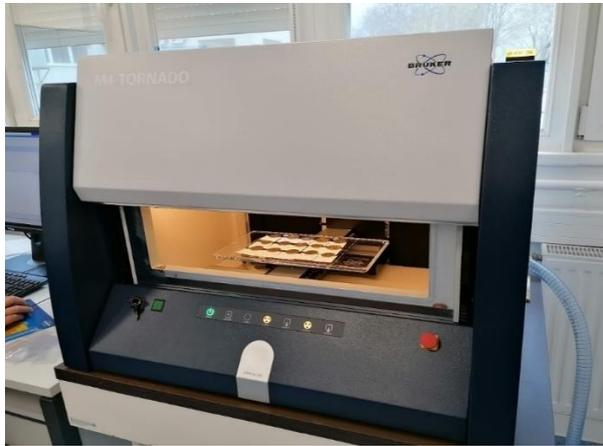
Fig 9: The Micro-XRF Spectrometers M4 Tornado
