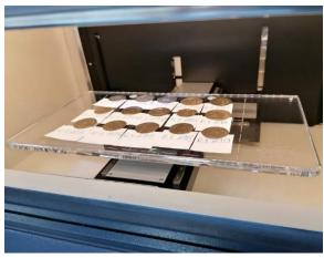
Fig 10: Analyzing dirhams form the Máramaros "Huszt" Hoard by Micro-XRF. (Photo: Al Halabi Suleman 2022)
