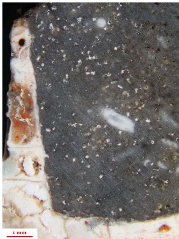
JM1A bedding mortar with greyish-black tessera. Dimensions of the tessera: 9 x 7 x 8 mm tessera embedded from the mosaic of Jado house,
