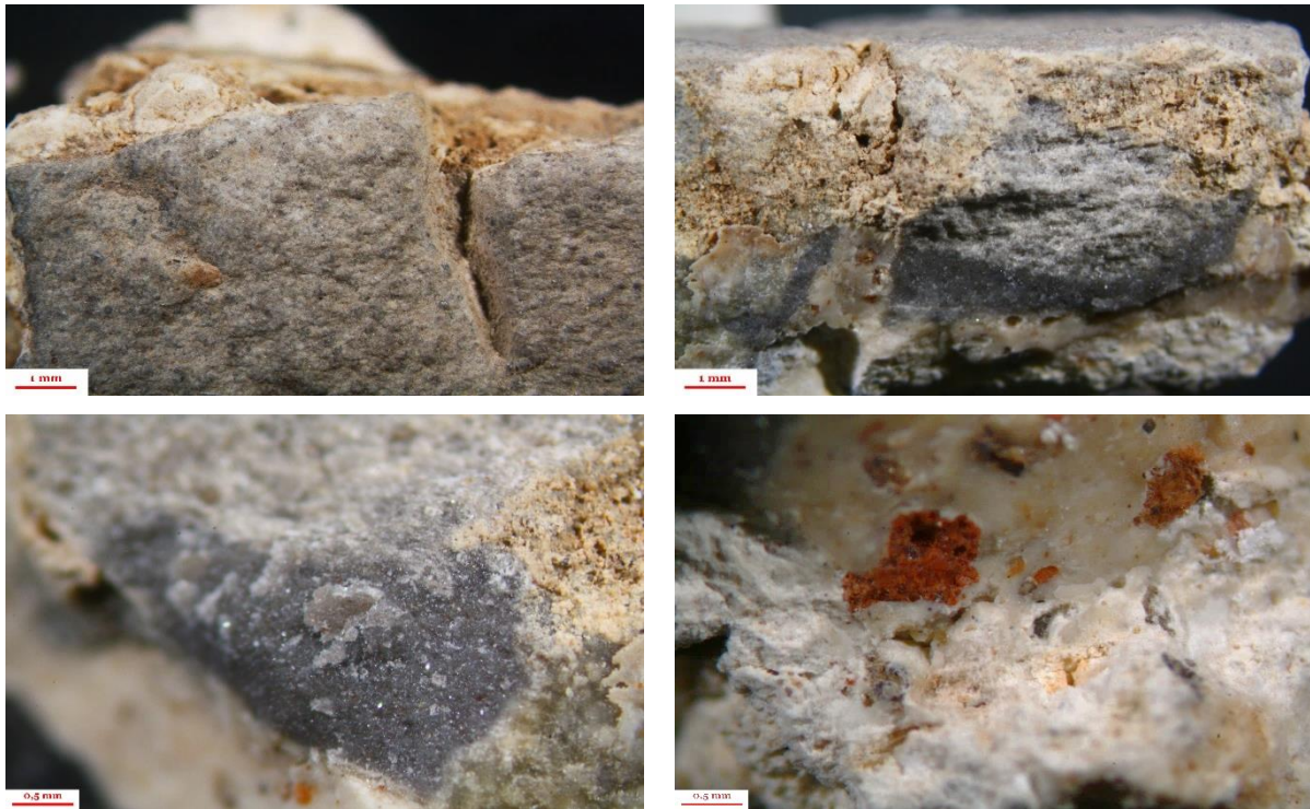
Fig 237. Photomicrographs of the sample JM11 of Two greyish black tesserae of the bedding mortar of Jādū al-Matnī house, Philippopolis, Syria, (analyse and photo: Brigitta Maria Kürtösi, 2022)
