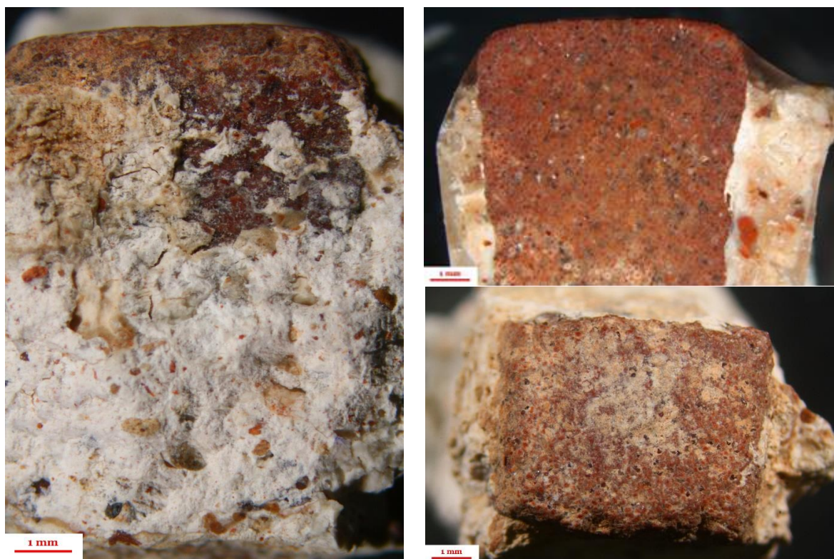
Fig 240. Photomicrographs of the sample JM7A of the Deep red tesserae in bedding mortar of the mosaic of Jādū al-Matnī house, Philippopolis, Syria, (analyse and photo: Brigitta Maria Kürtösi, 2022)
