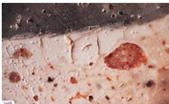
Fig 234. Photomicrographs of the cross section of the sample JM1A of the greyish-black tessera in the bedding mortar of the mosaic of Jādū al-Matnī house, Philippopolis, Syria, PLM VIS, PLM UV (analyse and photo: Brigitta Maria Kürtösi, 2022)
