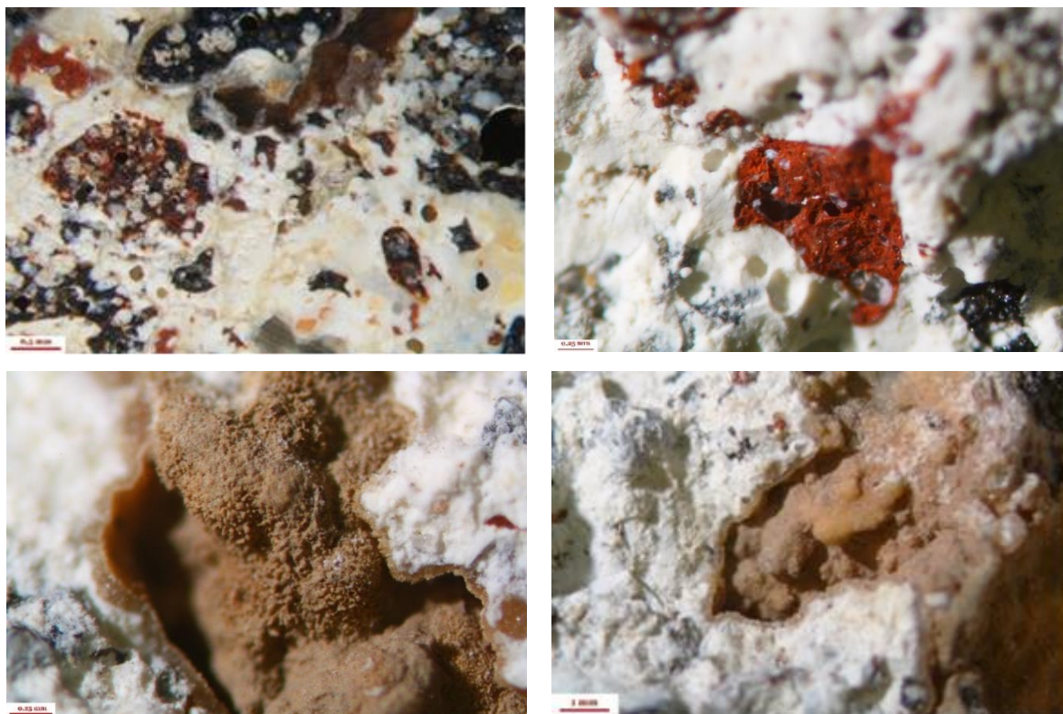
Fig 229. Photomicrographs of the raw sample and the polished cross section of KM3/Rudus or 2nd nucleus layer of al-Qabbānī house mosaic, Philippopolis, Syria, (analyse and photo: Brigitta Maria Kürtösi, 2020)
