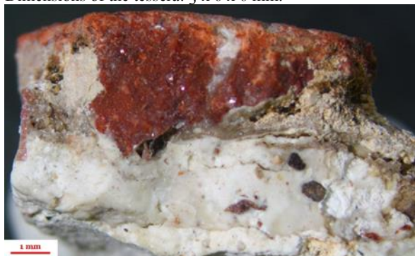
JM9 bedding mortar with red tessera. The height of the tessera is 3 mm. Stereomicrographs of bedding mortar samples with
