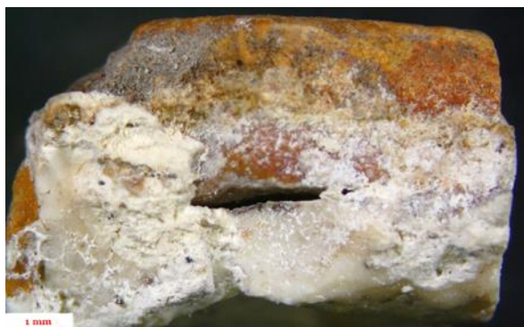
JM4B yellow tessera in bedding mortar Dimensions of the tessera: 3 x 6 x 6 mm.
