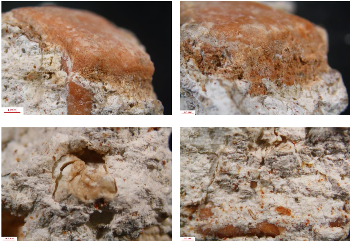
Fig 242. Photomicrographs of the sample JM8 of the Pink tessera in bedding mortar of the mosaic of Jādū al-Matnī house, Philippopolis, Syria, (analyse and photo: Brigitta Maria Kürtösi, 2022)
