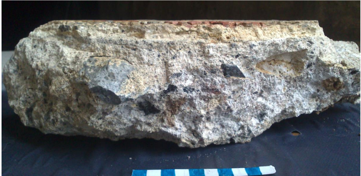
Fig 202. Part of the foundation layers of mosaic of the house of Jādū al-Matnī shown the used of less thickness tesserae, Philippopolis, Syria (photo: Maher Jbace 2014)
