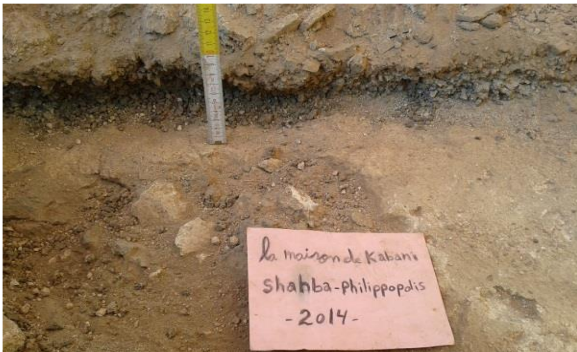
Fig 250. Atypical layer of black volcanic vesicles in the stratigraphy of the lime floors in al-Qabbānī house, Philippopolis, Syria (Photo: Osama Nofal, 2014)
