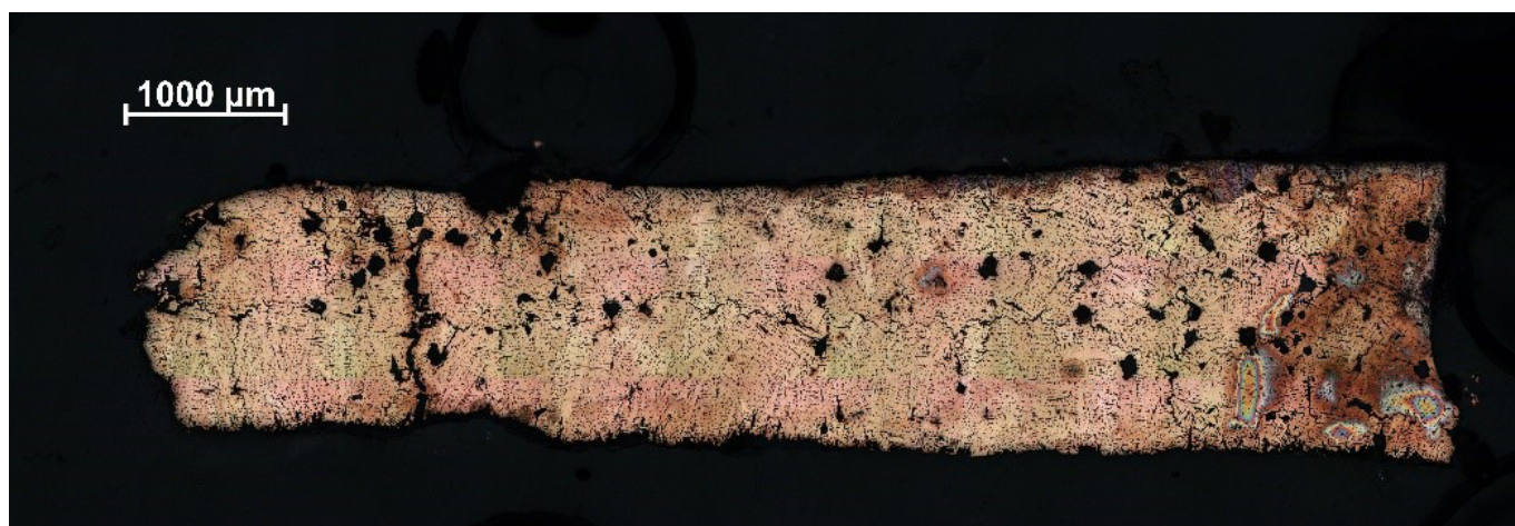
Fig. 2. OM-image of the microstructure of the sword-guard
